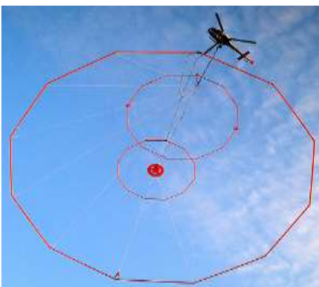
Geotech Ltd. VTEM Airborne Survey Array
